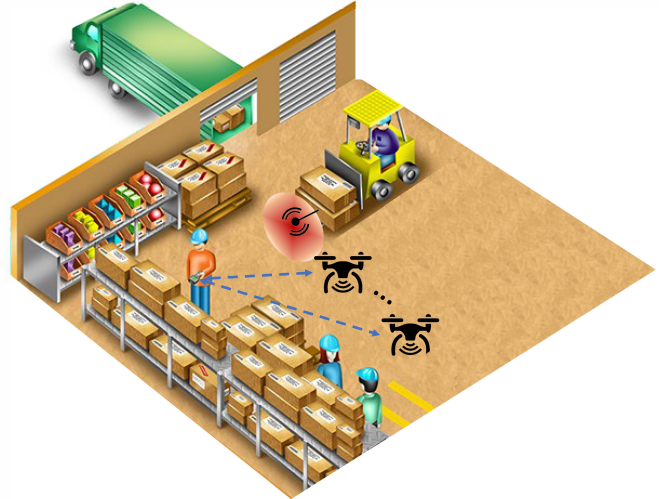
Fig. 2: Reference Scenario. While operating indoors, a drone tries to detect jamming (red color) in a low-BER regime, i.e., before the jamming affects the quality of the legitimate communication link (blue color).
