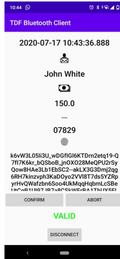
Fig. 8. Screen shown on the AAT to validate the transaction. \mathcal{A} can verify that the details of the intended transaction match the ones on the screen. Then, in case of Scenario #1 , \mathcal{A} can validate the transaction by pressing confirm . In case of Scenario #2 , \mathcal{A} can insert the code on the PAT to validate the transaction (see Figure 9.)
